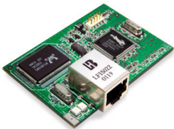
FIGURE 6 EMBEDDED INTERNET MODULE.
