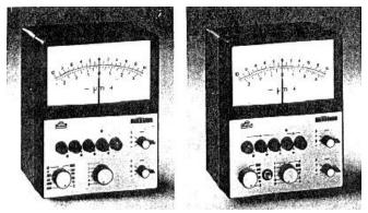
FIGURE. 4 Traditional instrument used as the basis for development of virtual instrument - Analog Millitron system (Mahr-Feinprüf).
