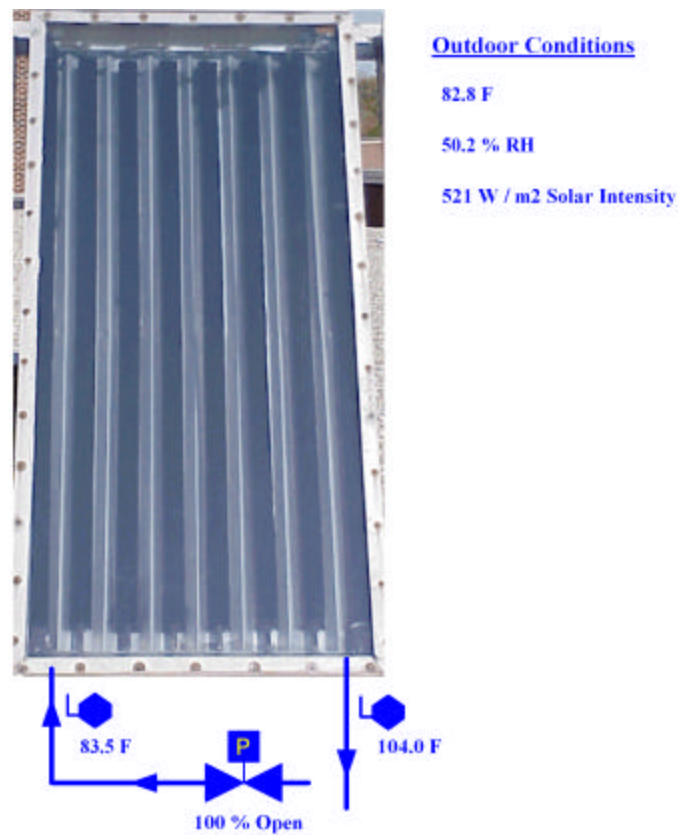
FIGURE 3. SOLAR COLLECTOR DATA IS ACCESSED OVER THE INTERNET USING A PROPRIETARY GRAPHIC INTERFACE .
