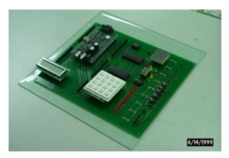
Fig.2 C50 DSK extension board layout
