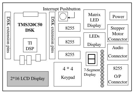
Fig.1 DSK50 Extension Board
