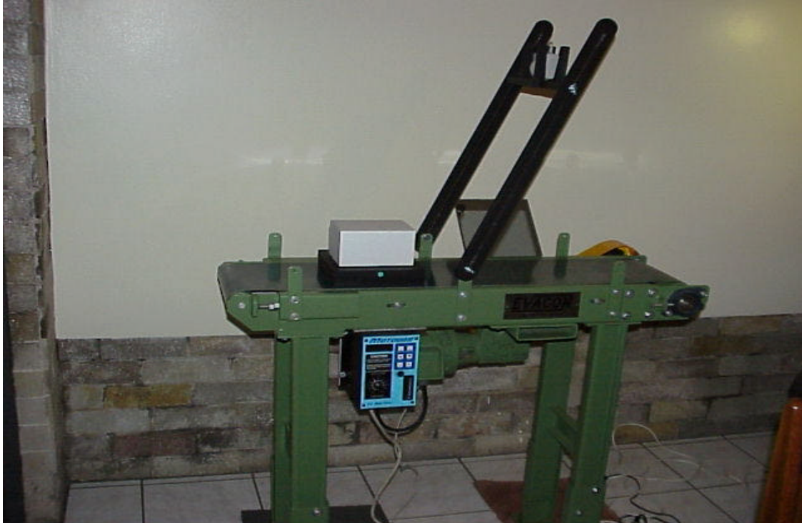
Fig. 4. The experimental setup, showing conveyor belt, camera, mirror and object.
