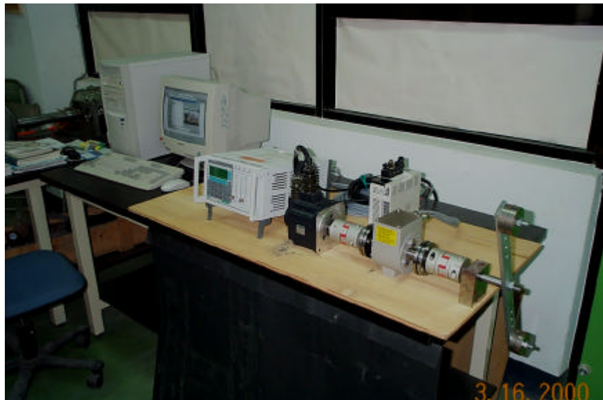
Figure 4 On the Controlling Servomotor by Motion Curve of the Simulated Cam
