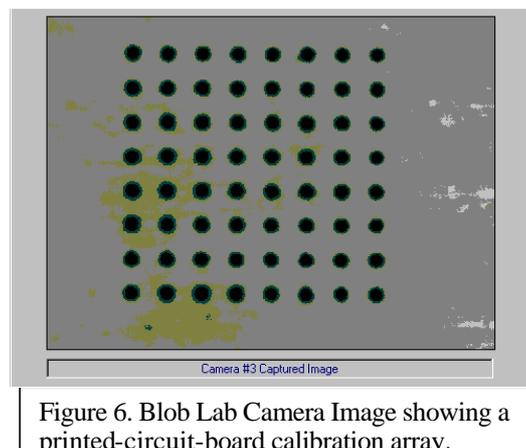
Figure 6. Blob Lab Camera Image showing a printed-circuit-board calibration array.
