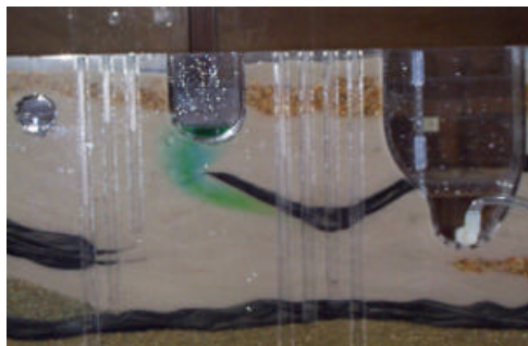
Figure 4. The pollutant infiltrates from the river.
