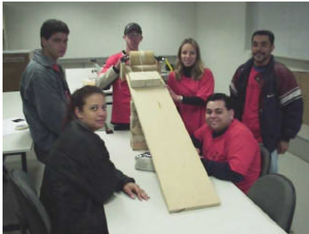
Figure 2. Members of the red team working on the experimental determination of the moment of inertia of a homogeneous wooden cylinder, as part of task 2.
