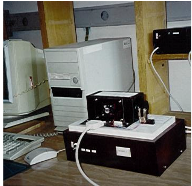
Fig. 4. View of the experimental laboratory stand HAA with external microcomputer measurement unit CTRL connected to PC and program support WinCTRL.
