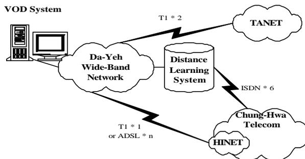
Fig. 5. The constructing VOD system in Da-Yeh University.
