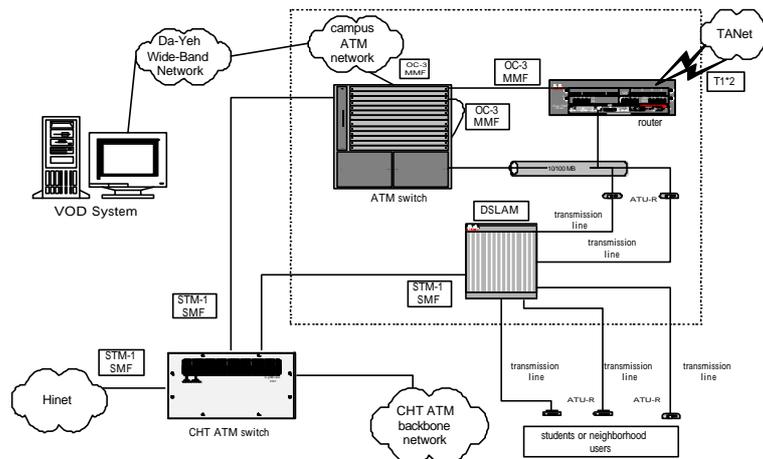
Fig. 6. The structure for the outgoing connection in the VOD system.
